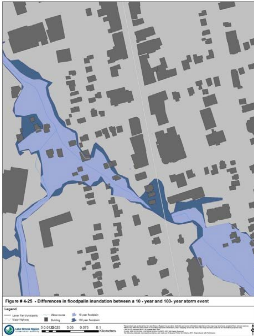
Figure 4-25 The difference in floodplain inundation between a 10-year and 100-year storm event
