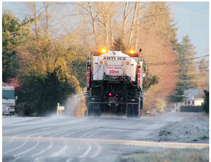
Figure 5. Truck applying brine to the road
