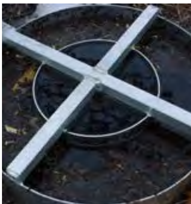
Left: BMP holding water longer than design drawdown time. Right: Double-ring infiltrometer.
