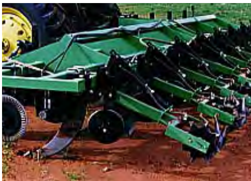
Deep Tilling: Greater than 30cm in depth (depth chisel plow, larger mechanical rototiller)
