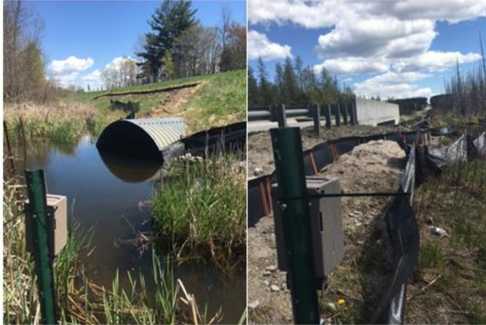
Figure 7. Trail cameras set to capture wildlife passing through the ecopassages (left) and using the artificial nesting structures (right)
