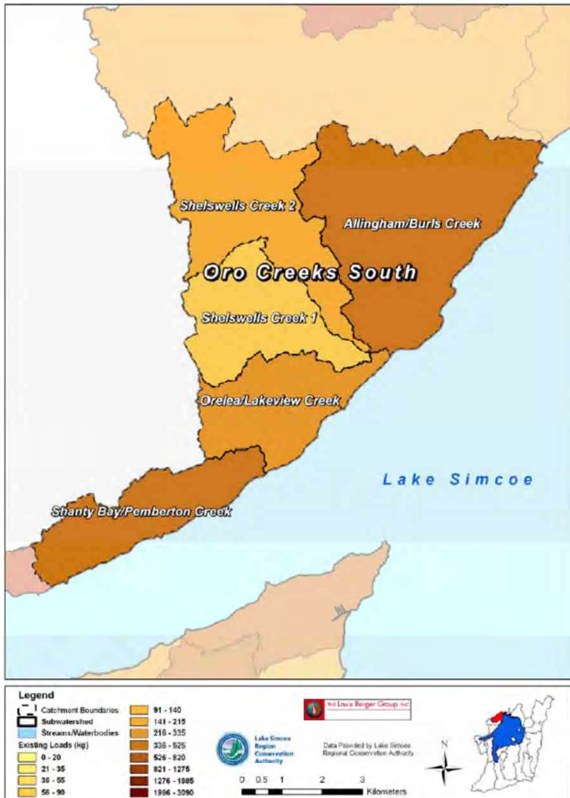
Figure 3-14: Oro Creeks South subwatershed agricultural BMP scenario total phosphorus loads (Louis Berger Group Inc., 2010).
