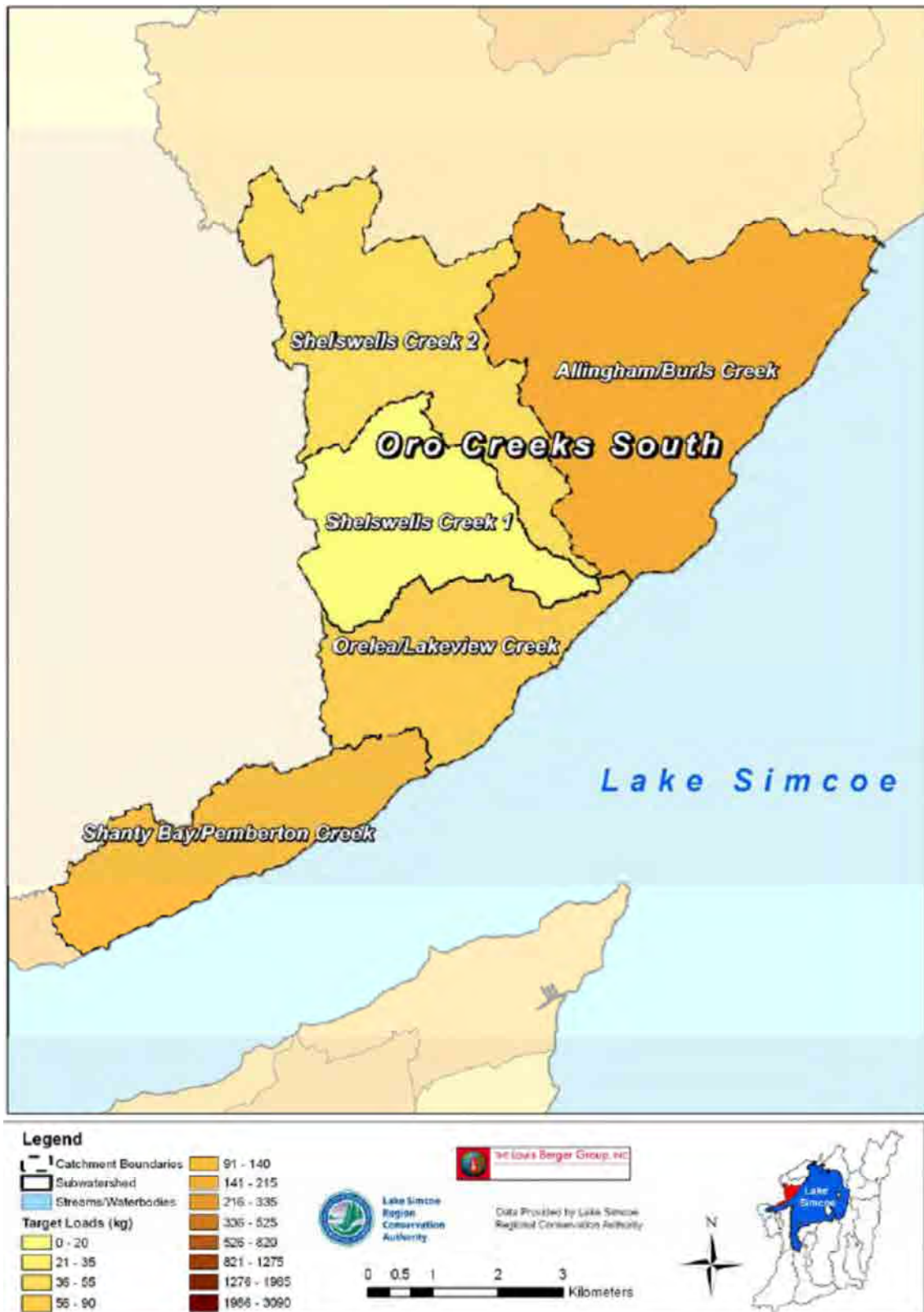
Figure 3-15: Oro Creeks South subwatershed target total phosphorus loads (Louis Berger Group Inc., 2010).
