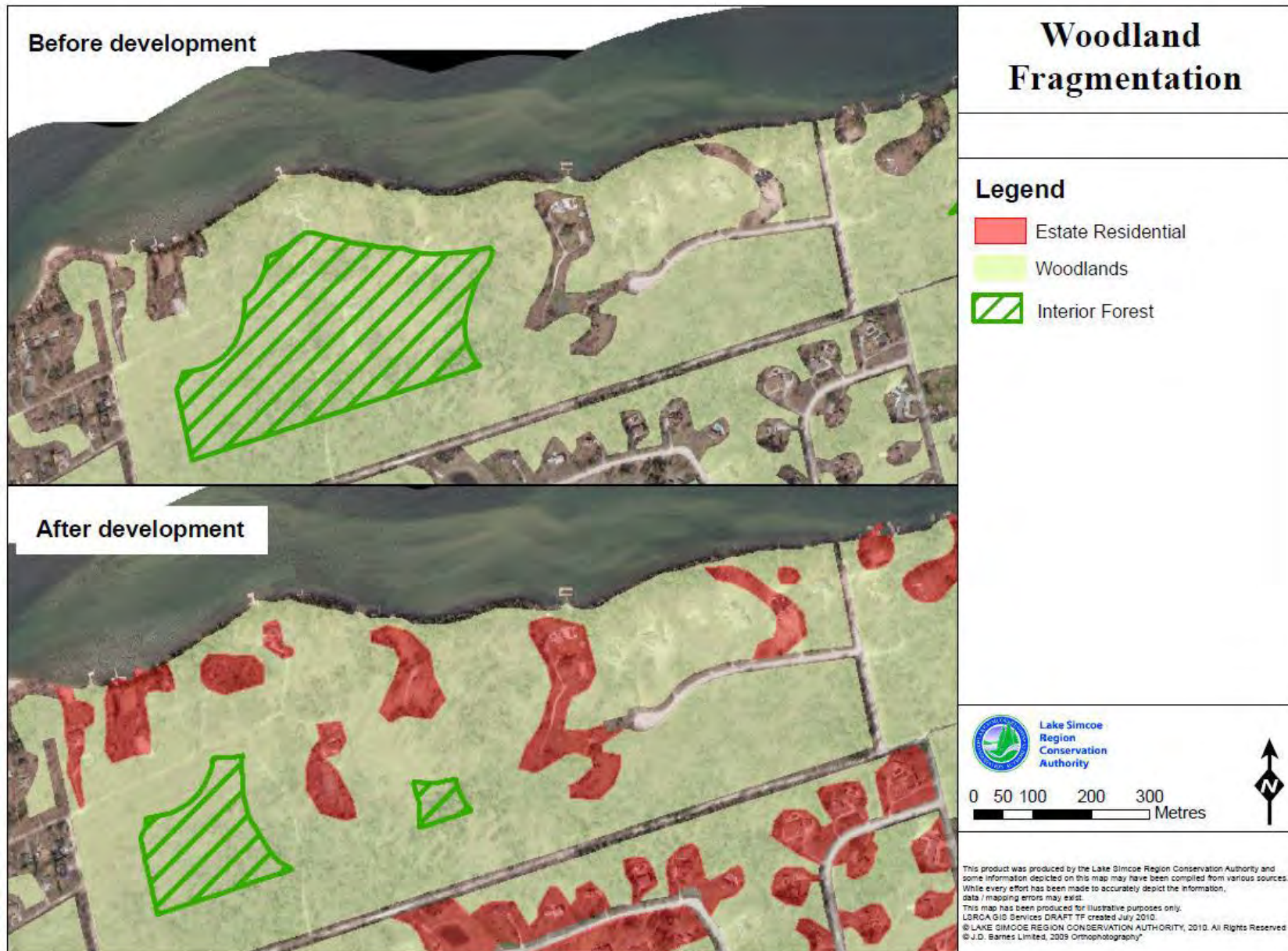
Figure 6-9 Example of loss of forest interior resulting from estate residential development
