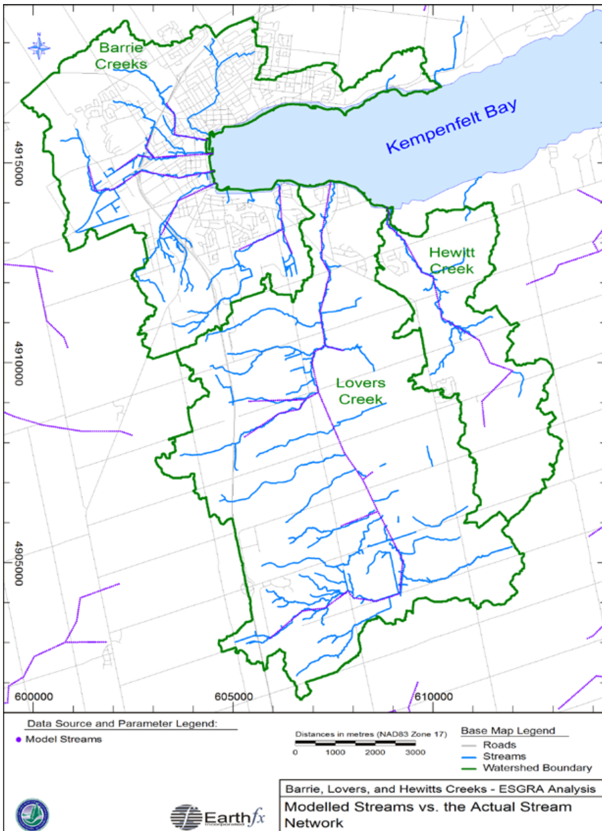
Figure 4: Comparison of the simulated streams versus the actual stream network. (Model = purple, MNR mapping = Blue). For Barrie creeks, please see Figure 5.
