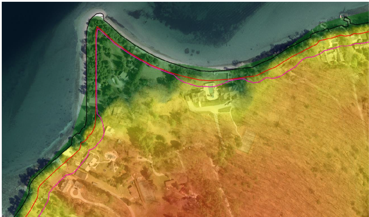
Figure 7.2: Example of Stable Slope Allowance in Variable Topography
