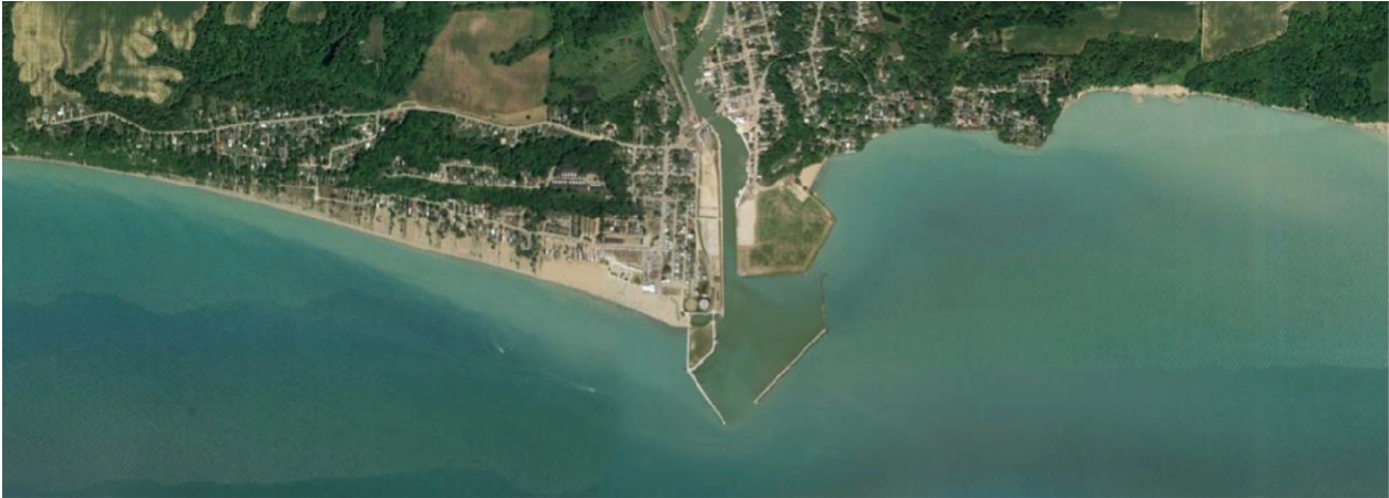
Figure 9.2: Disturbance in Alongshore Sediment Transport at Port Stanley, Lake Erie
