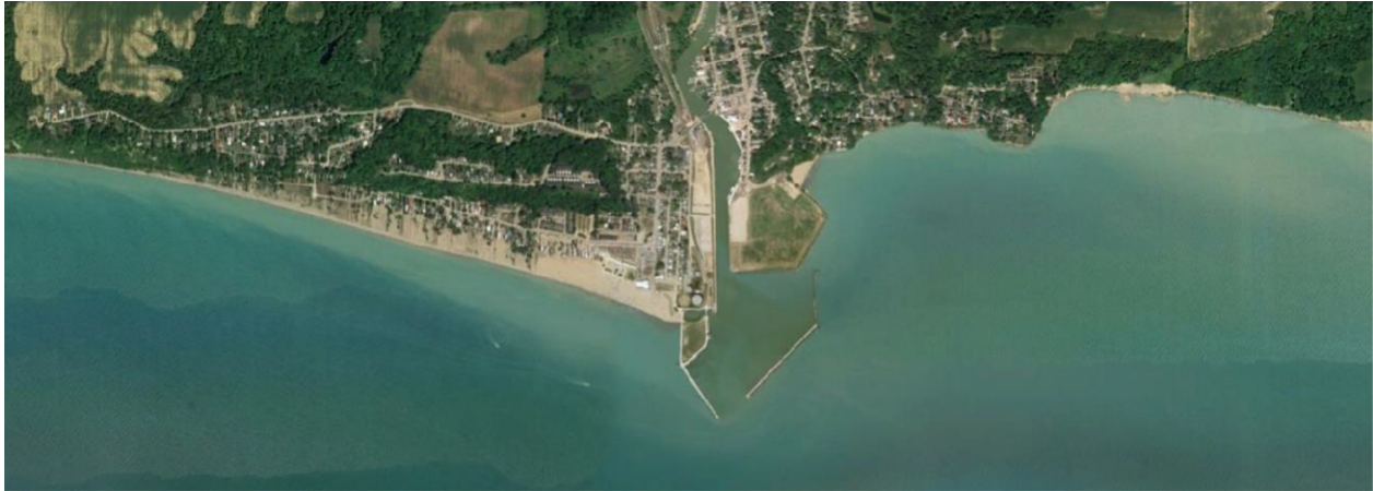
Figure 9.2: Disturbance in Alongshore Sediment Transport at Port Stanley, Lake Erie
