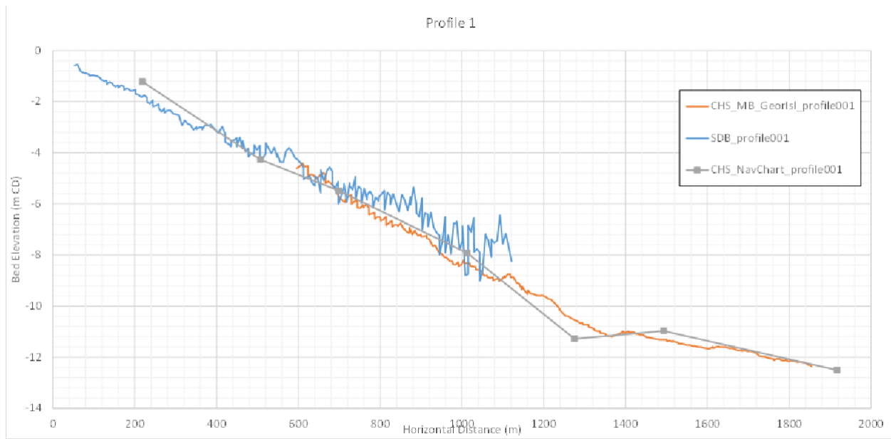
Figure 2.11: Comparison of CHS Multi-beam, CHS Point Data and SDB Bathymetric Data at Profile 1
